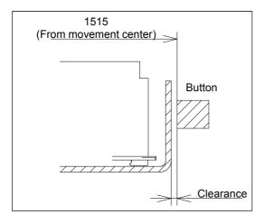
To keep the clearance, it is recommended to use button spring.
